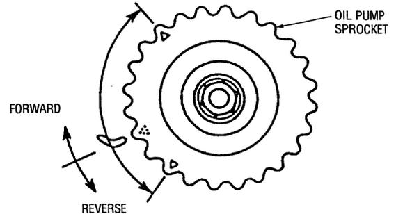
4. If the movable range of the oil pump sprocket exceeds the specified range, correct as follows:
