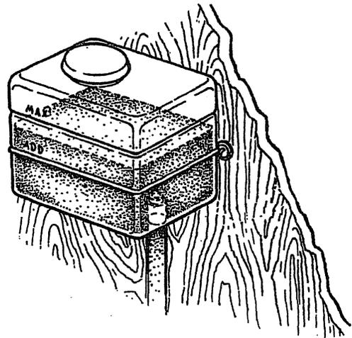
**NOTE:** This tank, with its short run of plastic hose, is best located at or above the level of the engine's exhaust manifold.
