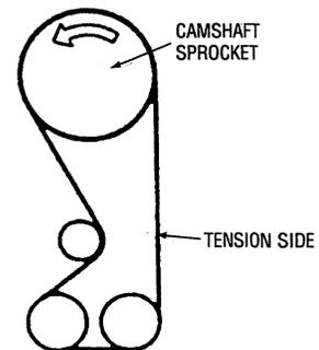
7. Loosen the temporarily tightened tensioner nut on the water pump side 1 or 2 turns, and tension the belt making use of spring force.
