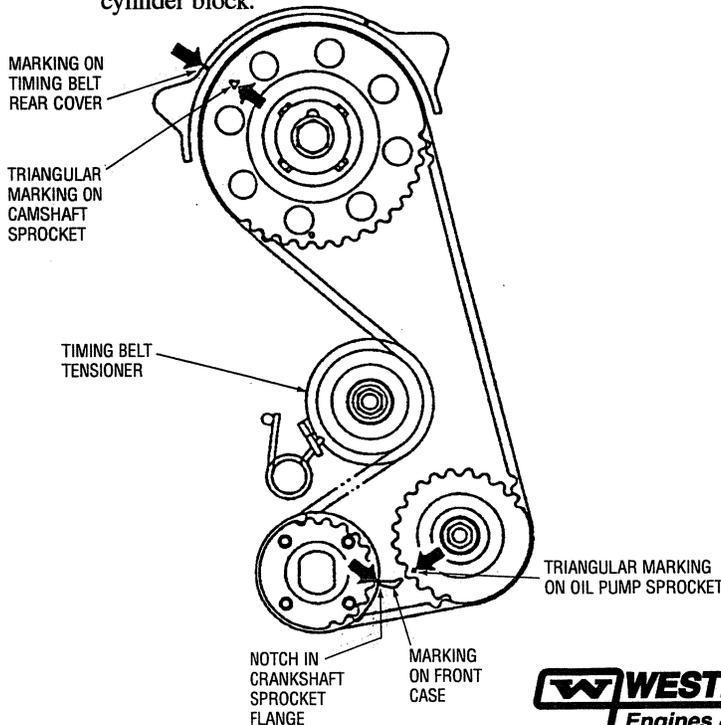
At this time, check that the moveable range of teeth on the oil pump sprocket is according to specifications.
