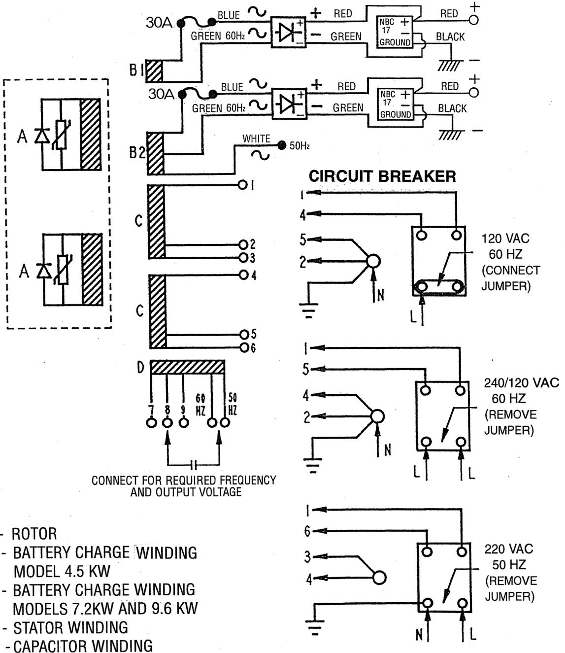
**⚠ WARNING:** When changing from 60Hz to 50Hz, make certain the ground wire (white & green stripe) is properly repositioned according to this diagram.
